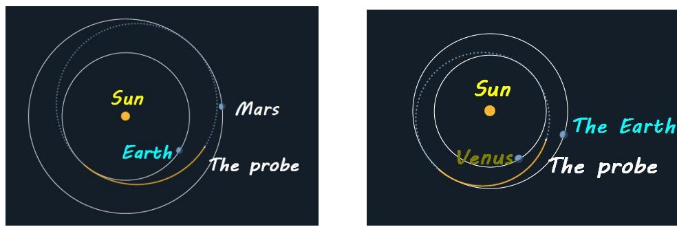
Figure 1: Transfer orbits between the Earth and another planet
