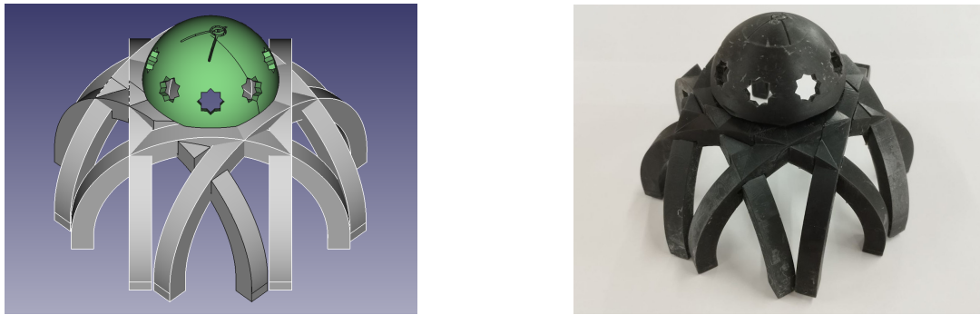
Figure 11: Complete model with interlocked arches and upper dome. Picture of the 3D printed model.
