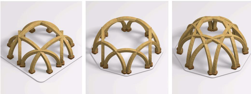
Figure 13. Rendering of the 3 types of ribbed domes: lattice + diamond, and stars [8/2] and [8/3].
